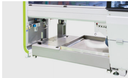
300/400 l tank without automatic filter
