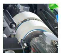
Grinding is followed by polishing for the ultimate in smooth, performance enhancing glide. Integrated in the Scout sdp model, the polishing module smoothes the edges right up to the tip of the ski.
