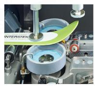
Do you want the edges to be perfect? Ceramic discs provide a higher quality, more precise edge than a belt. Consistent and precise.
