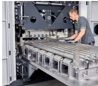
Advanced cleaning system for leveling rollers
