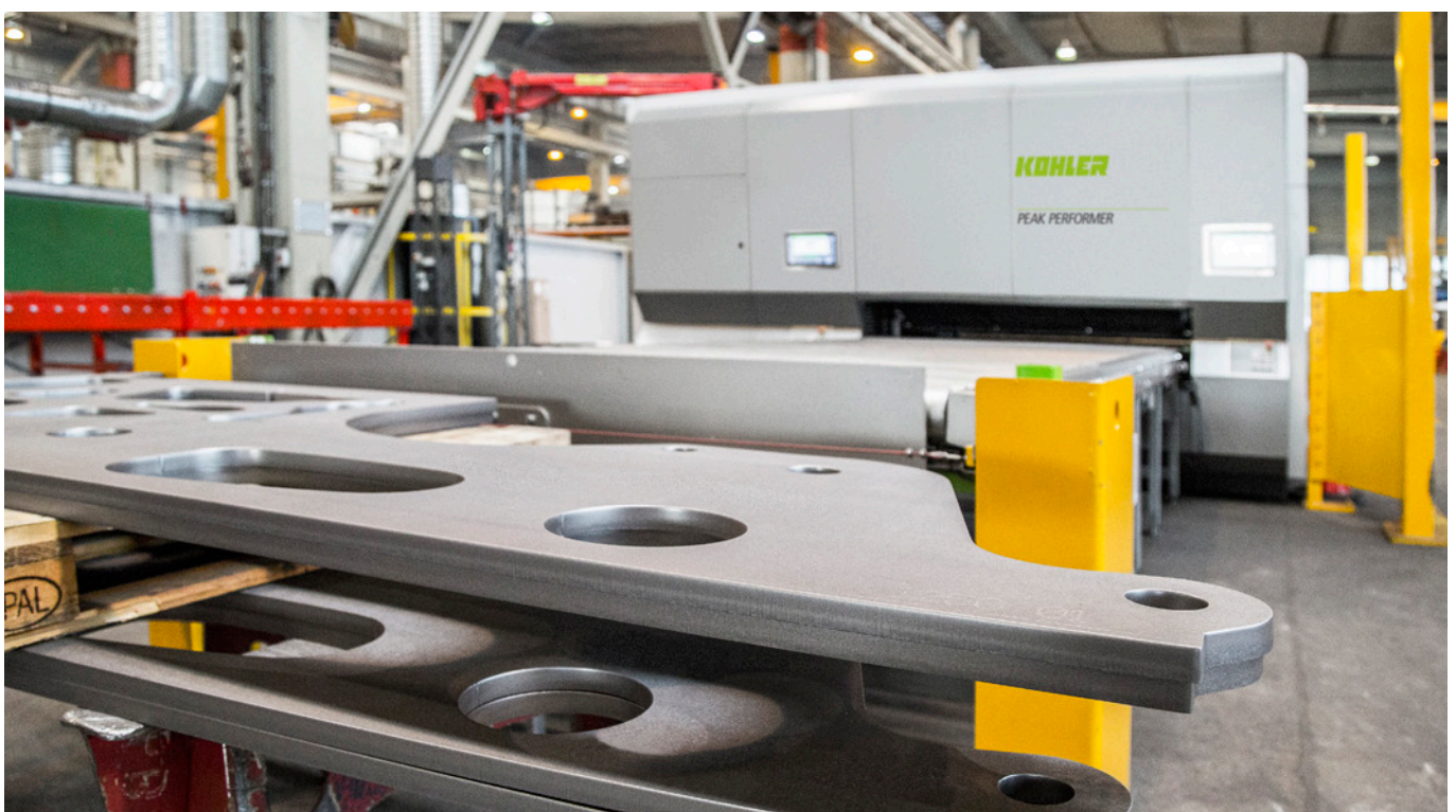
Compact precision leveling machine for manufacturing connectors
